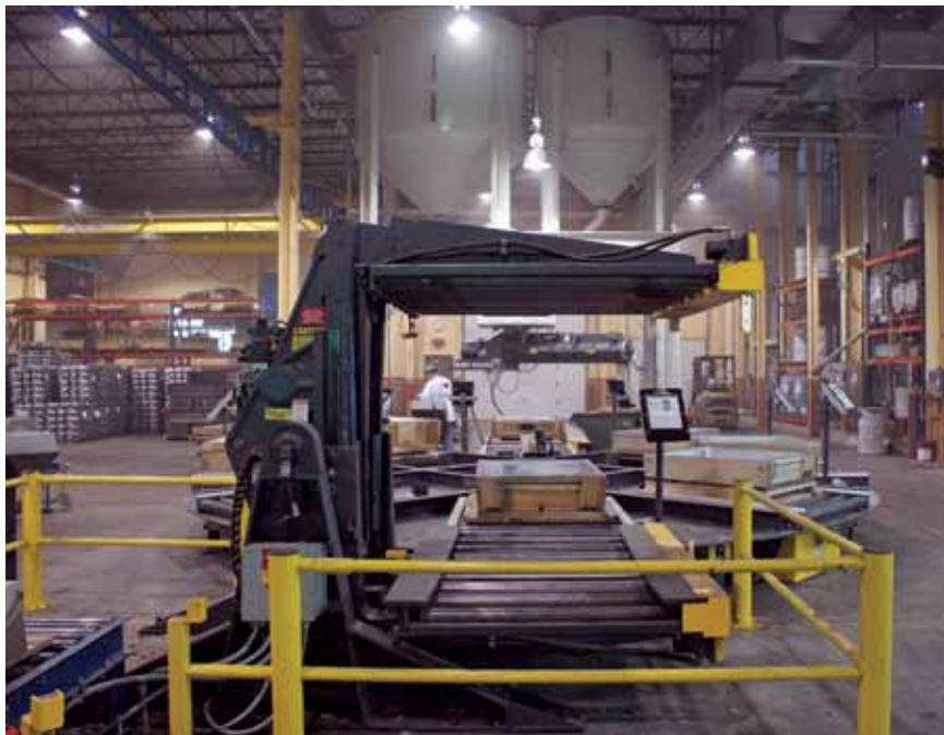
Olson utilizes a mold turntable in its new nobake line at its facility in Rockford, Ill.
