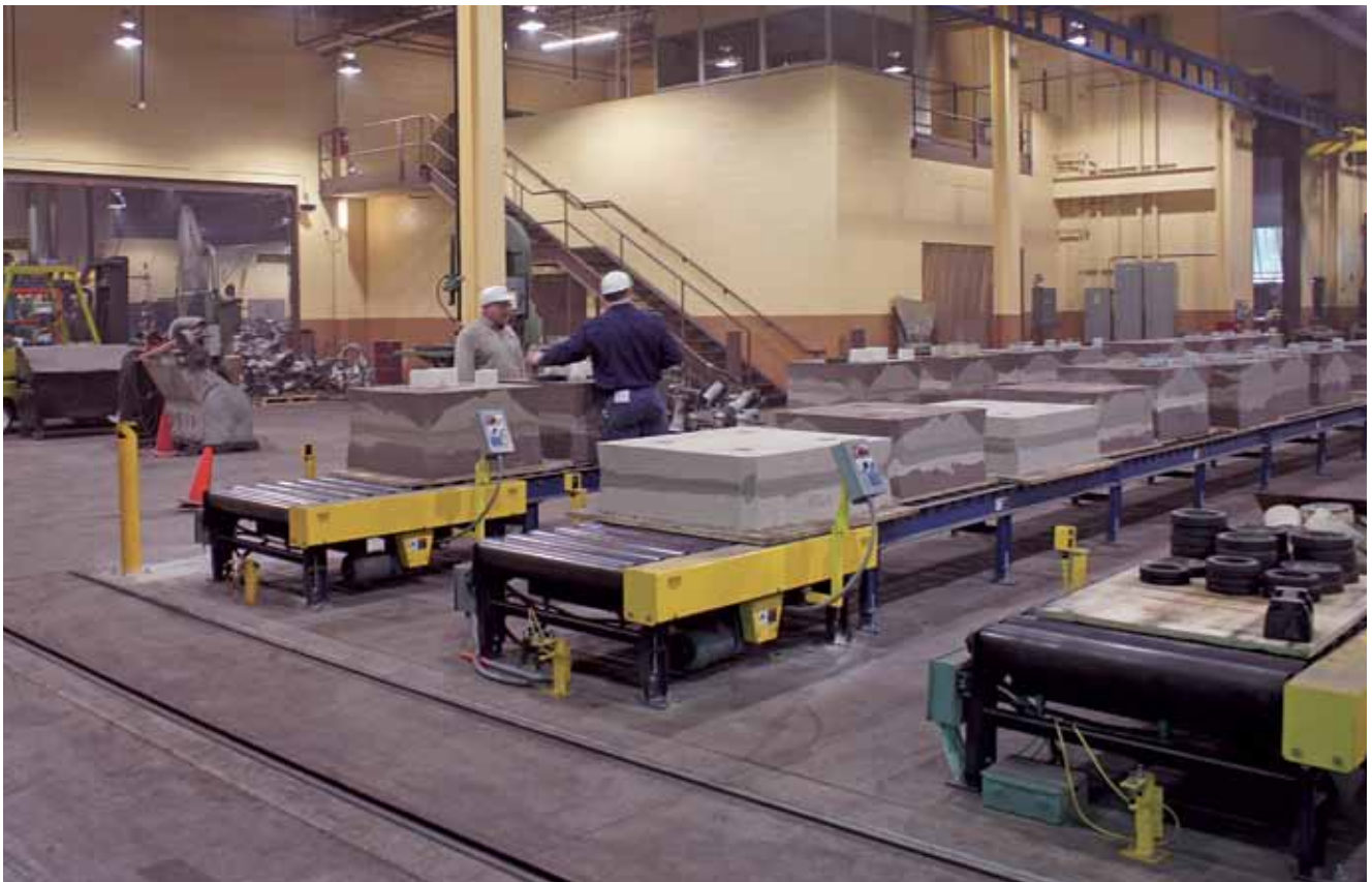
The nobake line will take on new jobs requiring larger dimensions, as well as function as overflow capacity for the Olson Aluminum's original green sand casting lines.
