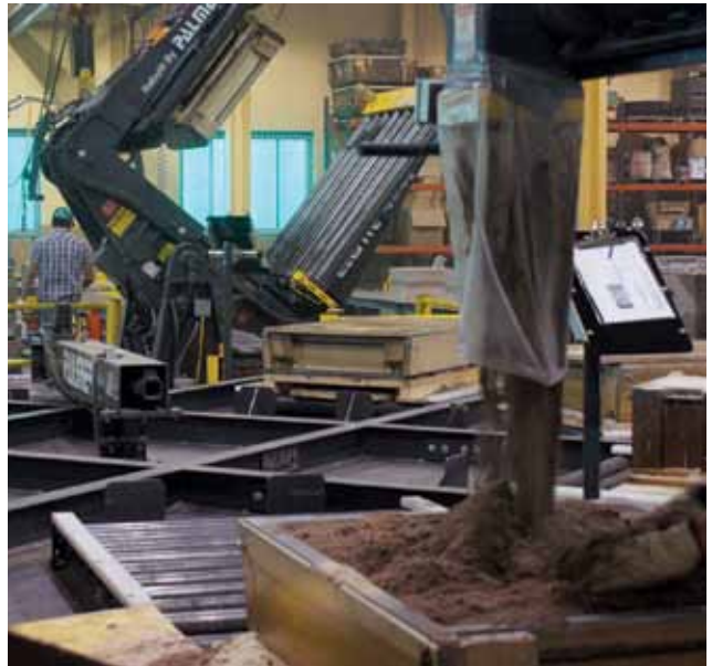
After nobake cope and drag molds are made, they are transferred via turntable to a machine that pairs the halves together.
